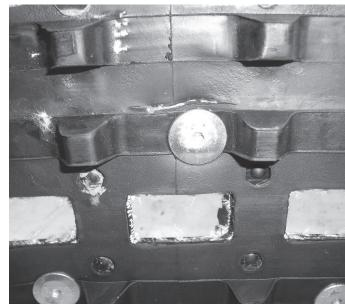
Torn belting generally caused from foreign objects, such as sticks, rocks, trailer edges, compromises track structural integrity and can lead to sudden track failure. It is recommended to replace track.
