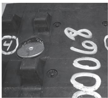
A traction stud tear-out generally results with a ripped hole in the track belting. This compromises track structural integrity and can lead to sudden track failure. It is recommended to replace track.
