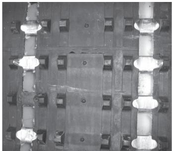
Missing and excessively worn track clips should be replaced before any further use. Replacement clips are available. Clip replacement cost should be evaluated 1st with customer with consideration to overall condition of the track. It may be more cost effective to replace track.
