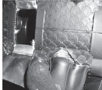
Outside lug wear and fatigue occurs with usage. Snow coverage conditions and track spin generally have the greatest impact. Track performance, such as traction, braking and overall stability is deteriorated with excessive lug wear and fatigue. It is recommended to replace track.
