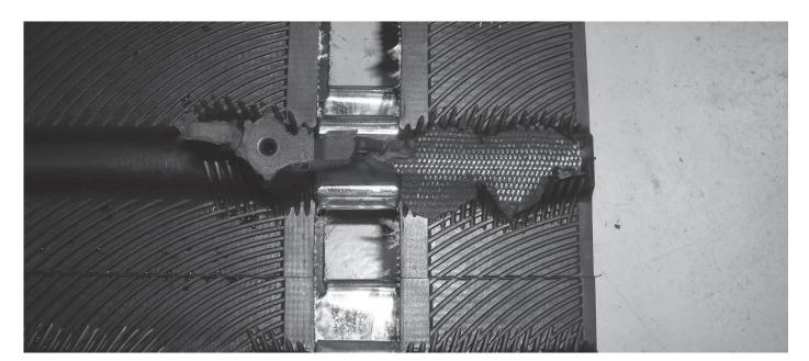
Torn and missing outside lugs occur with usage. Snow coverage conditions, contact with foreign objects, track spin, or using the wrong track design for riding style & terrain generally have the greatest impact. Track performance, such as traction, braking and overall stability is deteriorated with torn and missing outside lugs. It is recommended to replace track.
