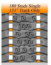
The Long Track Template 171 single pattern is used to create this 180 stud pattern. Read Tech Tip T7-12-0012
