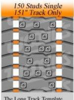
The Long Track Template 171 single pattern is used to create this 150 stud pattern. Read Tech Tip T7-12-0012
