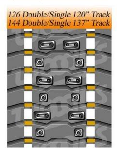
**Important**-- If installing Angled Digger® support plates, the hole(s) for drilling will be offset from the original pattern holes marked. Center the Angled Digger® support plate between the lugs over the original pattern marked. Create a new offset mark for drilling in the center of the hole of the Angled Digger® support plate. Refer to the Angled Digger® Support Plate Installation instructions included in the package.
